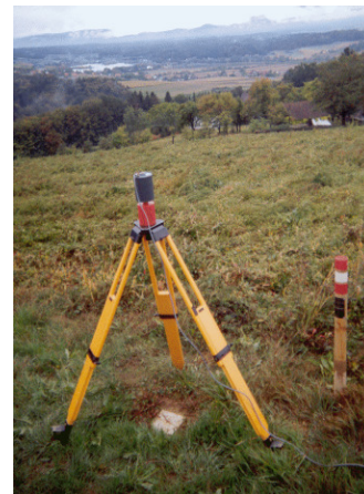
Figure 1: Repeat station site in Austria, Proton Magnetometer on tripod.
