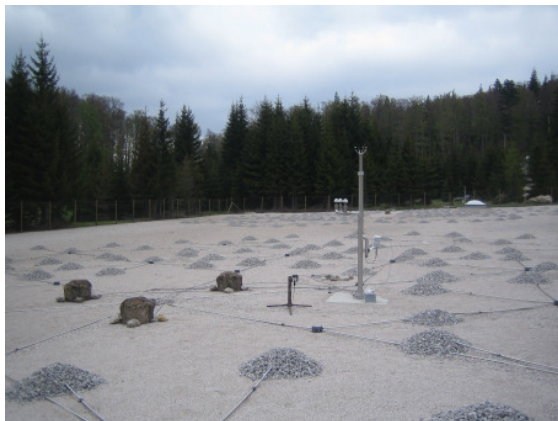
Figure 1: A multiple-inlet infrasound system at the Conrad Observatory with a reference-microphone triplet to the left.
