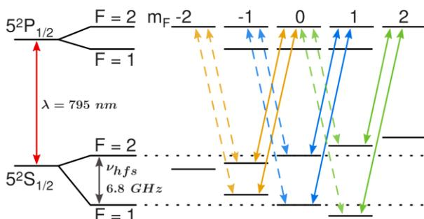
Figure 1: Excitation scheme of multiple  $\Lambda$ -systems within the hyper fine structure of the  $^{87}\text{Rb-D}_1$  line. The dotted and solid lines indicate resonances with different  $m_F$  quantum numbers.
