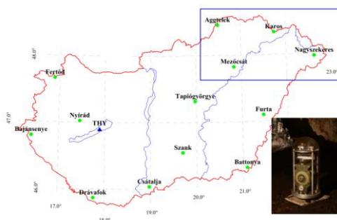
Figure 1: The Hungarian repeat station network (H-RS). The picture shows the on-site DIDD variometer installed near to Aggtelek station. The blue rectangle represents the area where the on-site recording is applied in the data reduction.
