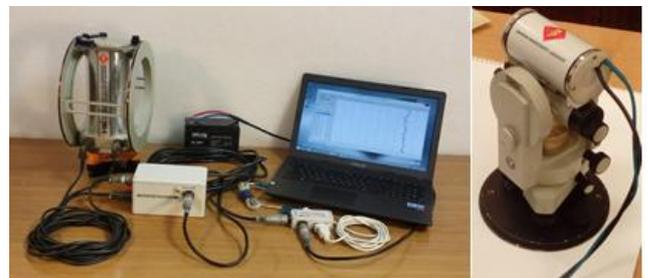
Figure 1: Vector magnetometer POS-4, POS-DIMOVER & non-magnetic theodolite
