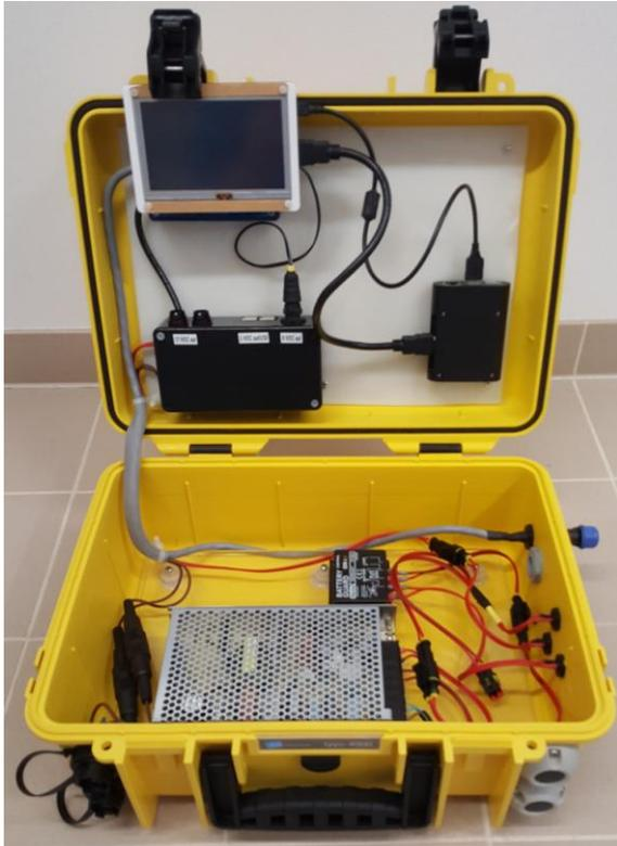
Figure 1: Connection box with mobile MARTAS system, unbreakable power supply (battery not shown), lightning protection, remote control.
