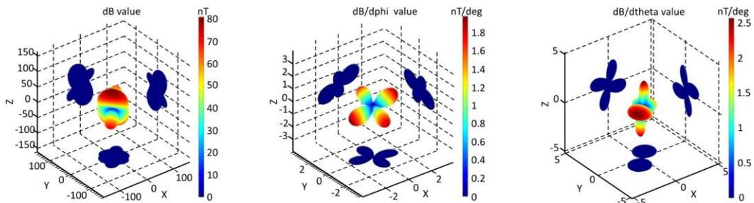
Figure: The possible  $\delta B$ ,  $\delta B/d\varphi$  and  $\delta B/d\theta$  errors at  $B=50000$  nT and simultaneous deviations  $\alpha_{12}=89.9^\circ$ ,  $\alpha_{23}=\alpha_{13}=90.1^\circ$ ,  $k_1=1$ ,  $k_2=1\cdot 10^{-4}$ ,  $k_3=1\cdot 10^{-3}$ .
