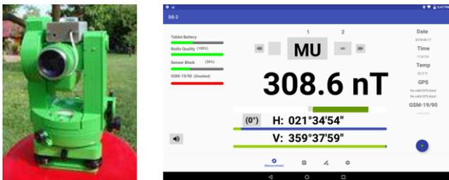
Figure 1: DS- 2 digital absolute instrument
