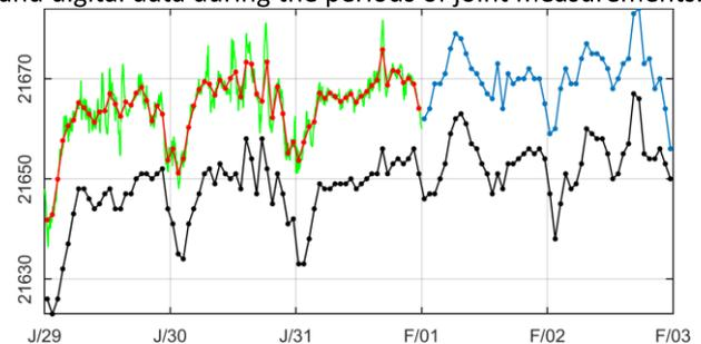
Figure 2: Example of filling of the gaps in the data of the observatory PET during 01-31 January, 1997 (horizontal component  $H$ , nT). Green curve—minute data obtained by digitization of the analog magnetograms (see Khomutov and Khomutova, 2016); red curve — hourly data calculated from minute values; blue curve — hourly values obtained by manual processing of magnetograms (from WDC); black curve — hourly data of observatory MMB (from WDC, for comparison).
