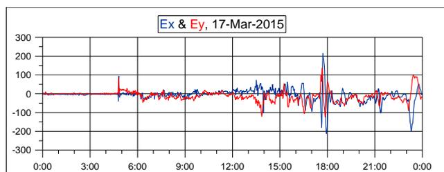
Figure 1: Plane wave model of horizontal components of geoelectric field based on the observations of geomagnetic field at Budkov Observatory on 17<sup>th</sup> March 2015
