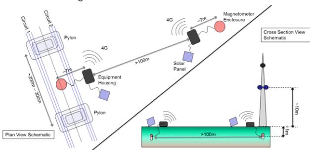
Figure 1: Schematic of the Differential Magnetometer System
