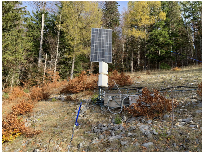
Figure 1: Fully installed monitoring system (solar panel, Geomon4D measuring boxes on the pole), aluminium boxes with fuel cell and batteries.
