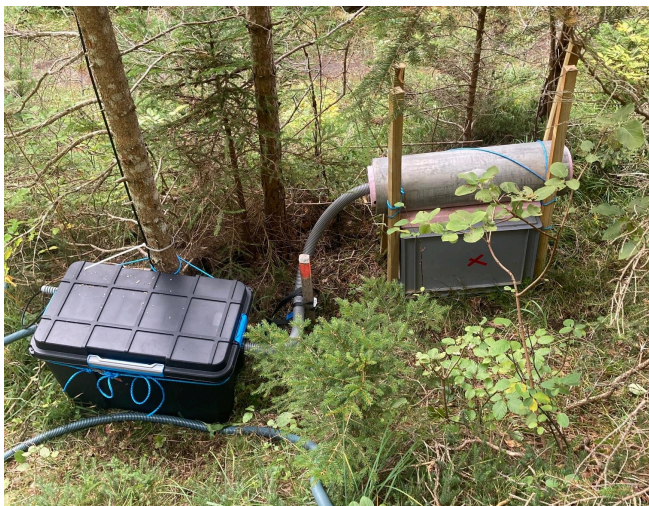
Figure 1: One of four stations under a high-voltage line. The Overhauser magnetometer is placed inside a thick aluminium cylinder (right) which acts as a shield against high-frequency disturbances. The black box (left) contains the electronics.
