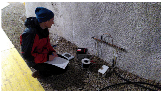
Figure 1: Copper wires coming out of the gravel connected by a bracket. Electric current is conducted from a lead battery over a small resistor into the grounding system. The other connection is on the other side of the main tunnel.
