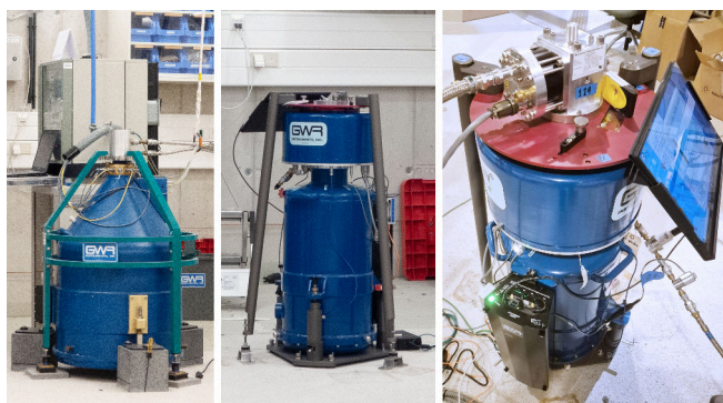
Figure 1: Left: the old GWR C025 (blue, foreground) with electronics (gray, behind). The green structure supports the cold head above the blue dewar. Middle: the new iGrav050 without cold head. The gray beams support the red plate on the top, on which the cold head is mounted. Right: the new iGrav050 in operation.
