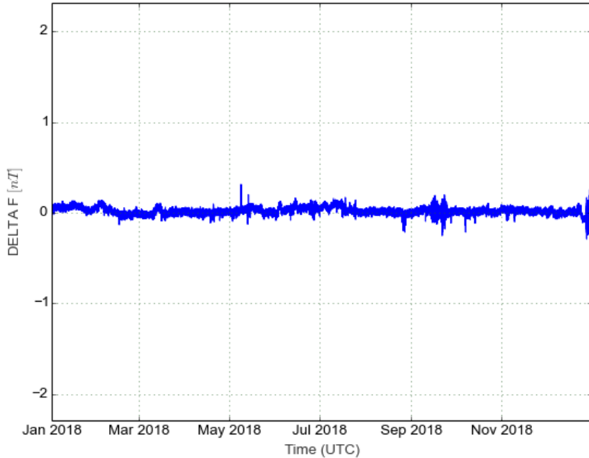
Figure 4.3: Delta F values between the scalar magnetometer and the field strength calculated from the baseline corrected vectorial data set. The scale of the figure is related to the INTERMAGNET 5 nT criteria.
