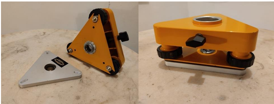
Figure 1. a) (left) The basement of the theodolite with baseplate already removed and the aluminium plate fixed to the pillar, b) (right) the theodolite basement installed on the fixed aluminium plate.
